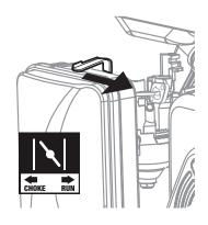
Allow the Engine to run for several seconds. Then, if the Choke lever is in the CHOKE position, move the Choke Lever very slowly to its RUN position.
